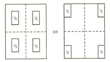
If a correction is not needed, proceed to the operating instructions. In a mechanical base, shift refers to the pivot distances of the levers. If, on a lever, the distances are equal, then a lever is said to have no shift error. Also, two levers which have the same ratio will have no shift error.
